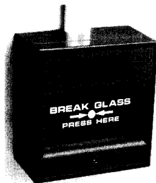
A call point, surface mounted on a Pattress, wired to two fire resistant cables to BS7629
